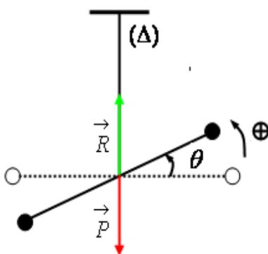
$$\text{تكتب المعادلة (*) : } -C.\theta = J_{\Delta} \frac{d^2\theta}{dt^2} \quad \text{أو : } \frac{d^2\theta}{dt^2} + \left(\frac{C}{J_{\Delta}}\right).\theta = 0 \quad (1)$$
